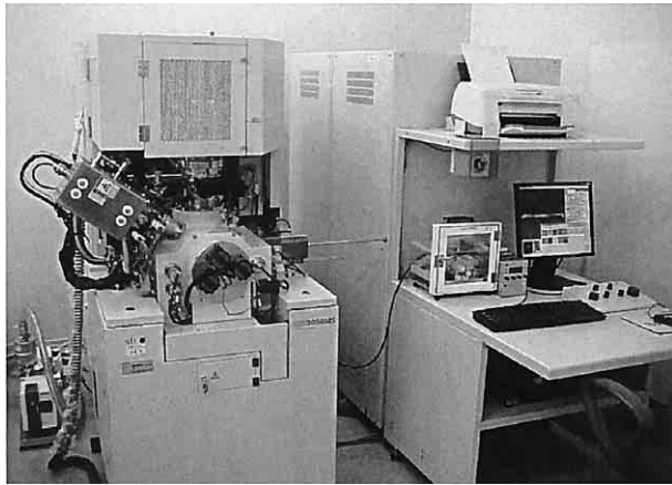
Photo 4 FIB-SEM (SII NanoTechnology Inc., SMI-3050MS2)
